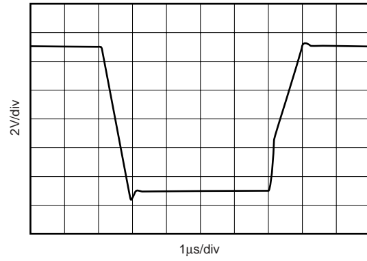
LARGE SIGNAL STEP RESPONSE ( G = -1\text{V/V} , R_L = 10\text{k}\Omega , C_L = 15\text{pF} )
