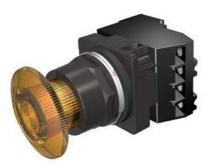
30mm BlackMax, Epoxy Coated Corrosion Resistant Complete Metal Unit Illuminated Twist-to-Release Transformer type, 480V AC Incandescent Lamp Mushroom Head Cap Small 1.79" (45 mm) Plastic Cap, Amber 2 Position Maintained, Twist-to-Release with 1 N.O. - 1 N.C. Heavy Duty Contacts, A600/P600 UL Listed, CSA Certified NEMA 1,3,3R,4,4X,12,13 & Automotive Standards
