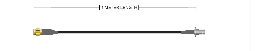
Connector A 132113 SMA Plug Straight Brass Gold + Heatshrink 50 Ohm RG-58 Continuity/Hi-Pot Connector B 112202 BNC Jack Straight Bulkhead - Rear Mount Brass Nickel + Heatshrink
