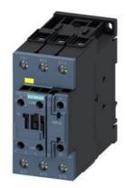
power contactor, AC-3e/AC-3, 65 A, 30 kW / 400 V, 3-pole, 83-150 V AC/DC, 50/60 Hz, with integrated varistor, auxiliary contacts: 1 NC, screw terminal, size: S2, F-PLC-IN
