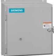
Non-reversing motor starter, Size 2 1/2, Three phase full voltage, Solid-state overload relay, OLRelay amp range 25-100A, 24VAC 50-60HZ coil, Non-combination type, Enclosure type 12, Dust/drip proof for indoors, Extra-wide enclosure
