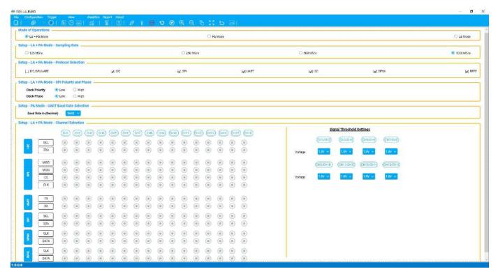
Users can easily configure the Logic Analyzer for embedded interfaces by either selecting Logic Analysis (LA) mode or Protocol Analysis (PA) mode or a combined (LA+PA) mode. This ensures a quick and easy way to configure the product and look at complex problems at system level either in Logic Analysis (State Analysis, Timing Analysis) or Protocol decoding or both. Save and Recall capability ensures designers can recall their custom setup details.
