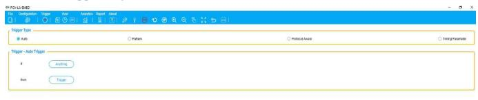
PGY-LA-EMBD supports Auto, Pattern, Protocol Aware and Timing Parameter trigger capabilities. Users can trigger on any of the Protocol packets. Comprehensive Trigger provides the flexibility to monitor different conditions.
