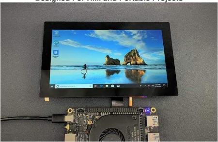
We have made many product design optimizations for HMI and portable project requirements. For example, HMI scenarios are often complex and dusty, but this display uses a fully fit design to perfectly prevent dust from entering the screen, and also effectively reduces the reflection of light. In order to make the screen easy to be installed, the screen edge comes with the special double-sided adhesive tape, which can be easily and firmly fixed.
