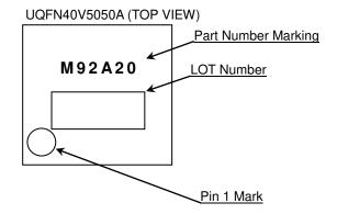
**Physical Dimension and Packing Information** Package Name UQFN40V5050A 5.0±0.1 0±0 1PIN MARK 00000000 0.035 -0:015 (0.203) 0.085 CO. 2 3.6±0.1 40 Detail A 3 0.4±0. 0.082 31 0  $\Delta$ 30 0.2±0.05 0.4 (U I NT : mm) PKG: UQFN40V5050A Drawing No. EX001-0014 <Tape and Reel information> Tape Embossed carrier tape 2500pcs Quantity Direction The direction is the 1pin of product is at the upper left when you hold reel on the left hand and you pull out the tape on the right hand of feed
