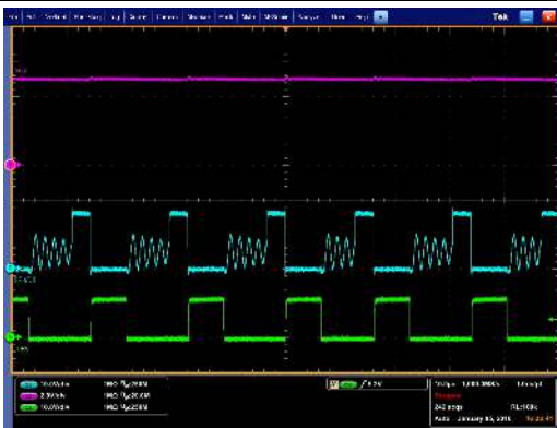
CH2 (Blue): Drain of synchronous rectifier Q1, 10V/Div CH3 (Mag): V_{OUT} , 2V/Div CH4 (Green): DRV signal to Q1, 10V/Div
