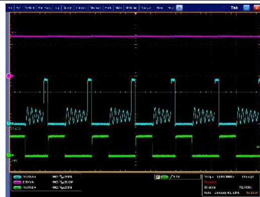
CH2 (Blue): Drain of synchronous rectifier Q1, 10V/Div CH3 (Mag): V_{OUT} , 2V/Div CH4 (Green): DRV signal to Q1, 10V/Div
