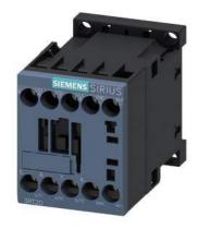
power contactor, AC-3e/AC-3, 12 A, 5.5 kW / 400 V, 3-pole, 24 V DC, with integrated varistor, auxiliary contacts: 1 NC, screw terminal, size: S00  $\,$
