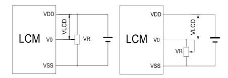
$V_{DD^{\sim}}V_{0}\text{: }LCD\text{ }Driving\text{ }voltage$
