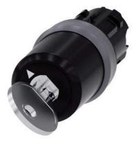
key-operated switch Siemens, 22 mm, round, plastic with metal front ring, special lock, with 2 keys, 2 switch positions O-I, latching, actuating angle  $90^\circ,\,10:\!30h/13:\!30h,$  key removal I
