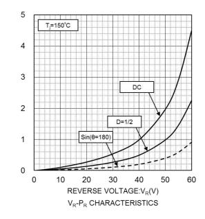
REVERSE POWER DISSIPATION:P<sub>R</sub>(W)
