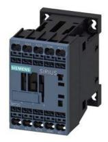
power contactor, AC-3 12 A, 5.5 kW / 400 V 1 NC, 24 V DC with diode integrated, 3-pole Size S00, Spring-type terminal
