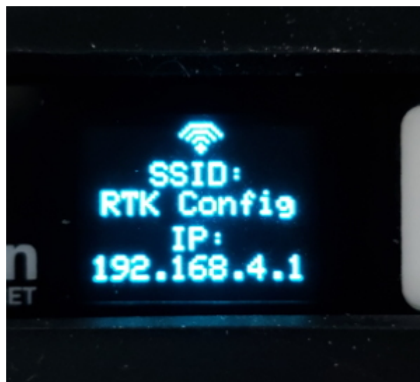
Device ready for cellphone configuration
