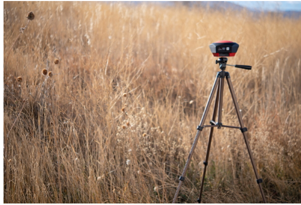
Temporary RTK Facet Base setup
