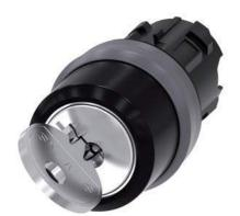
RONIS key-operated switch, 22 mm, round, plastic with metal front ring, lock number SB30, with 2 keys, 2 switch positions O<I, momentary contact type, Actuating angle 45°, 10:30h/12h, key removal O, possible special locks: SB31, 421, 455, with laser labeling, upper case and lower case, always upper case at the beginning of the word
