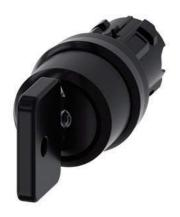
Key-operated switch O.M.R, 22 mm, round, plastic, lock number 73034, black, with 2 keys, 3 switch positions I>O<II, momentary contact type, actuating angle 2x45°, 10:30h/12h/13:30h, key removal O, with laser labeling, lower case
