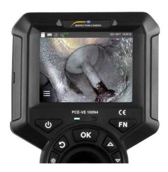
4-way industrial borescope with photo and video recording / 1280 x 720 pixels / 360° swivel / 6 mm (0.23") diameter / 1 meter (3 ft 2") cable length / LED lighting / Micro-SD card memory / Transport case / Battery life > 3 hours / IP 67
