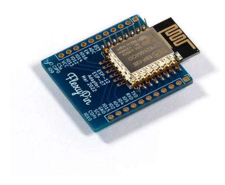
This board allows you to use various modules with a breadboard (and more) without having to solder the module in place. Just add FlexyPins
