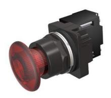
30mm BlackMax, Epoxy Coated Corrosion Resistant Complete Metal Unit Illuminated Push-Pull Operator Transformer type, 600V AC Incandescent Lamp Mushroom Head Cap Small 1 3/4" (44.5 mm) Plastic, Red 2 Position Maintained, Pull-to-Release UL Listed, CSA Certified NEMA 1,3,3R,4,4X,12,13 & Automotive Standards
