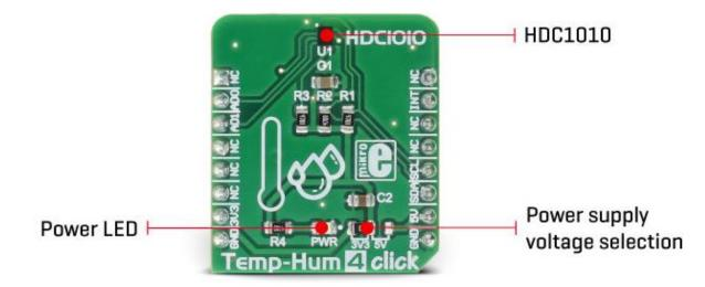
Internally, two sensors are connected to the ADC section, which can be set to sample the measurement with the resolution of 9, 11 or 14 bits, based on the measurement time. OTP memory holds the calibration coefficients that are applied to the measured value and the results are stored on the output registers, in the MSB/LSB format. These values are then used in formulas found in the HDC1010 datasheet so that the final temperature or relative humidity data can be calculated.
