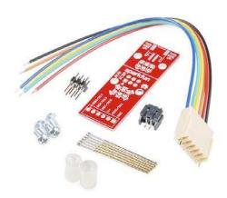
**Description:** Pogo pins make life so much easier when you are trying to program without having to solder a single thing, and when you attach them to an In-system programming (ISP) adapter they become instantly better, this simple kit allows you to do just that. Introducing the ISP Pogo Adapter, a simple and easy way to adapt pogo pins to a 6-pin ISP header allowing you to program an IC still without soldering a header to do so.
