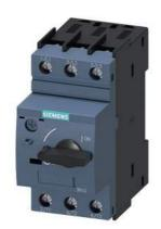
Special type Circuit breaker size S0 for motor protection, CLASS 10 A-release 34...40 A N-release 480 A screw terminal Standard switching capacity Ambient temperature -50  $^{\circ}\text{C}$  500 switching cycles
