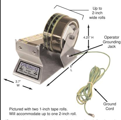
\*Best practice is grounding via supplied ground cord. Attach cord to snap on chassis and to common point ground. If grounded via placing on a grounded ESD worksurface, resistance to ground (RTG) should be periodically tested <1 x 10E9 ohms.
