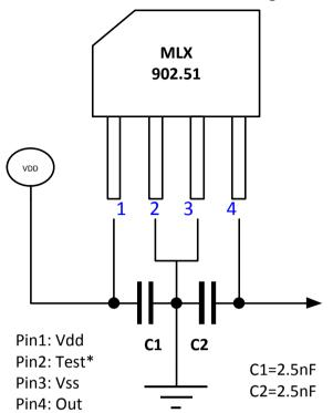
\*Readback diagnostic use only. Pin2 is not for programming device. For best results tie to Vss. Position Programmable Linear Hall Effect Sensor
