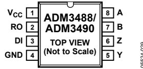
Figure 5. ADM3488/ADM3490 Pin Configuration
