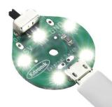
The PCB is designed to fit inside a 28mm square area, with the power switch in a position for ease of access. The board has a centred mounting hole to fit a standard M3 bolt. The LEDs are set on a 72° degree separation from each other, arrayed around the mounting hole.
