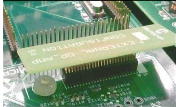
FIGURE 1: EXTERNAL OP AMP CONFIGURATION BOARD
