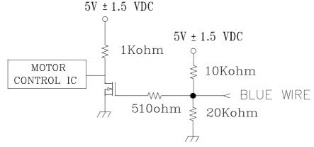
13-1. THE FAN SPEED WILL DEFAULT TO MAXIMUM WHEN THE SPEED CONTROL INPUT IS LEFT UNCONNECTED.
