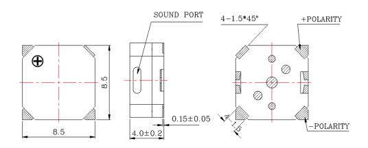
General tolerance =  $\pm 0.3$  mm and all measurements in mm unless otherwise noted.
