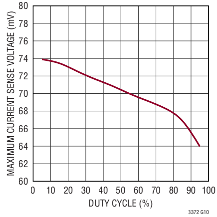
Maximum Current Sense Threshold vs Duty Cycle
