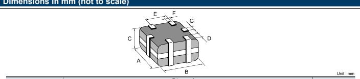
Part No. Dimensions Mass (Weight) (mg/pc.) (inch size) В С D Ε F G EXC24CS (0504) 1.25 ± 0.15 1.00 ± 0.15  $0.50 \pm 0.10$  $0.20 \pm 0.15$  $0.55 \pm 0.10$  $0.30 \pm 0.10$  $0.20 \pm 0.10$ 2.4
