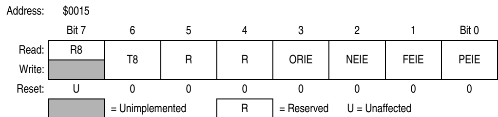
Figure 19-11. ESCI Control Register 3 (SCC3)
