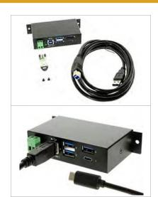
USB C hub provides 4 USB 3.1 Gen1 ports to include 3 USB-A ports and 1 USB C port. An ideal mini hub for super-speed data transfer in industrial environments! The USB C hub is a generation 1 hub of USB 3.1 supporting Super-Speed 5Gbps data transmission speeds and the reversible type-C port. This hub is self powered with a 2-pin terminal block connector to supply power input of +7  $^{\sim}$  48V DC sold separately.
