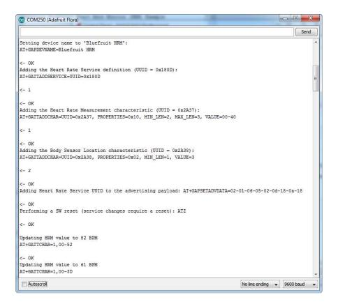
If you open up an application on your mobile device or laptop that support the standard <u>Heart Rate Monitor Service</u> (), you should be able to see the heart rate being updated in sync with the changes seen in the Serial Monitor:
