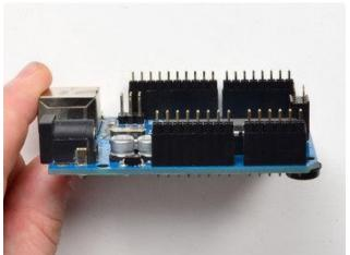
Also place the 2x3 female socket header into the ICSP header on the right of the board
