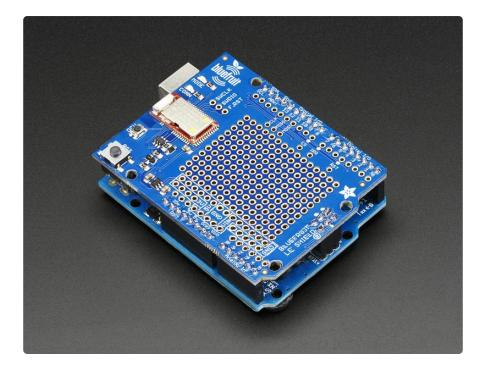
Would you like to add powerful and easy-to-use Bluetooth Low Energy to your robot, art or other electronics project? Heck yeah! With BLE now included in modern smart phones and tablets, its fun to add wireless connectivity. So what you really need is the new Adafruit Bluefruit LE Shield for Arduino!
