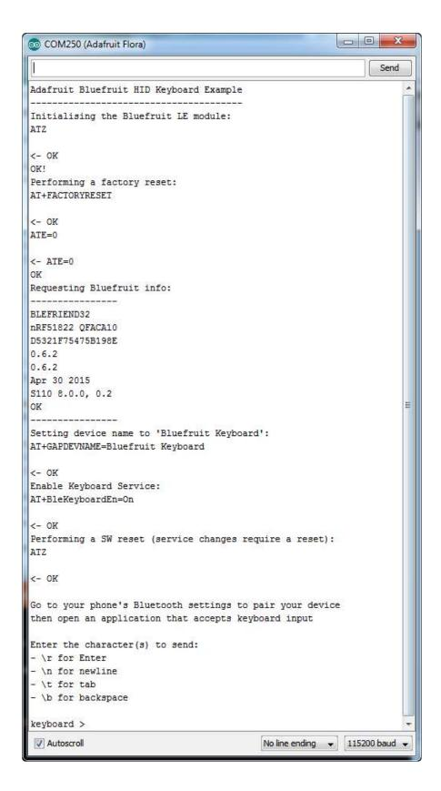
To send keyboard data, type anything into the textbox at the top of the Serial Monitor and click the Send button.
