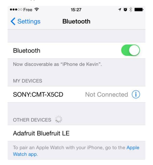
Once the bonding process is complete the device will be moved to the MY DEVICES category, and you can start to use the Bluefruit LE module as a keyboard:
