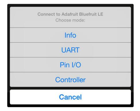
This will bring up a list of data points you can send from your phone or tablet to your Bluefruit LE module, by enabling or disabling the appropriate sensor(s).
