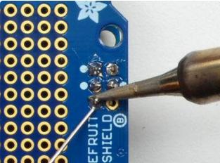
Don't forget the 6-pin socket!
