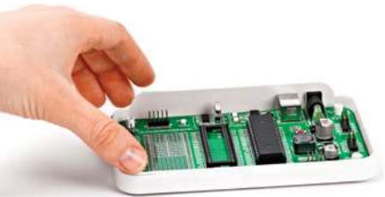
Figure 9-1: Integrating the board with the casing
