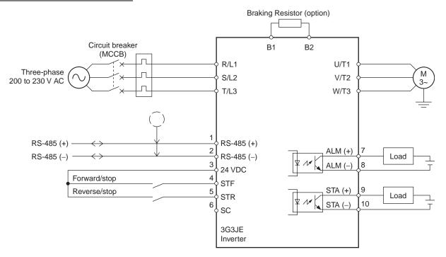
Note: The Braking Resistor (option) can be connected only to models with braking resistor control.
