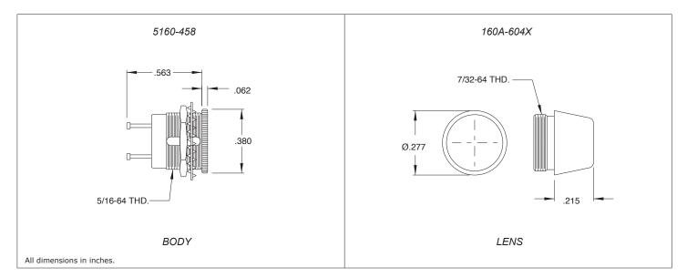
The Chicago Miniature Lamp Gemlite Indicator Light is a versatile design capable of accepting all T-1 sub-midget flange based lamps. These high quality indicators provide reliable service in a vast array of military and commercial applications where a miniature relampable front panel indicator is required. The lamp is not included with this indicator light. Please order the required lamp separately.
