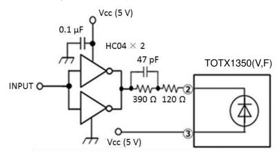
Replace 47 pF of capacitor with 82 pF if need a smaller jitter.
