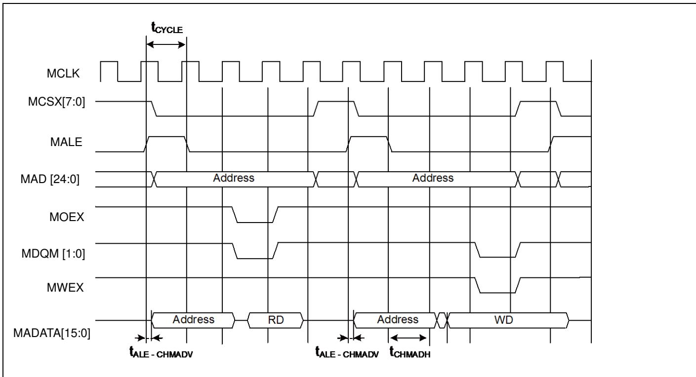
**Multiplexed Bus Access Synchronous SRAM Mode**
