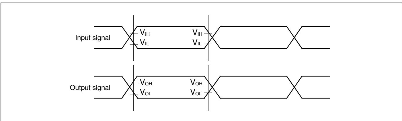
**Separate Bus Access Asynchronous SRAM Mode**
