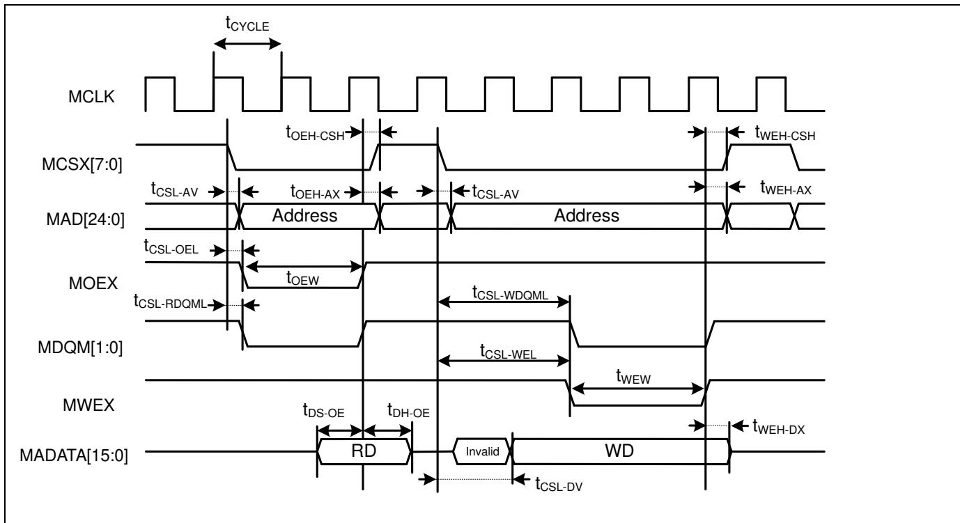
**Separate Bus Access Synchronous SRAM Mode**
