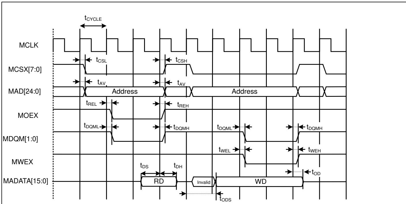
**Multiplexed Bus Access Asynchronous SRAM Mode**
