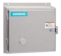
Non-reversing contactor, Size 1 3/4, Three phase full voltage, Contactor amp rating 40A, 3 wire (NO aux included), 24VAC 50-60Hz coil, Non-combination type, Encl NEMA type 4X 304 S-Steel, Water/dust tight noncorrosive, Extra-wide enclosure
