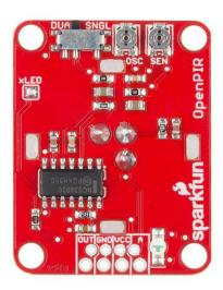
**Description:** The SparkFun OpenPIR is a highly customizable Passive Infrared (PIR) sensor based around the NCS36000 PIR controller. Passive infrared (PIR) sensors are able to detect motion in a small/local area — they're the sensor of choice in security systems, home automation and proximity-sensing applications. The OpenPIR allows you to set the sensitivity, trigger time and pulse mode of the motion sensor so you can tailor-fit it to your application!
