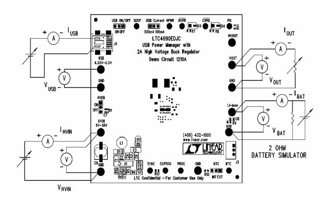
Figure 1. Proper Measurement Equipment Setup
