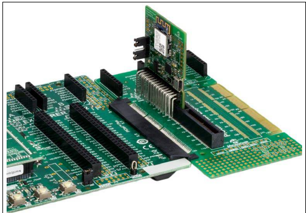
FIGURE 3-3: WINC1500 DAUGHTER BOARD PLUGGED INTO EXPLORER 16/32 DEVELOPMENT BOARD
