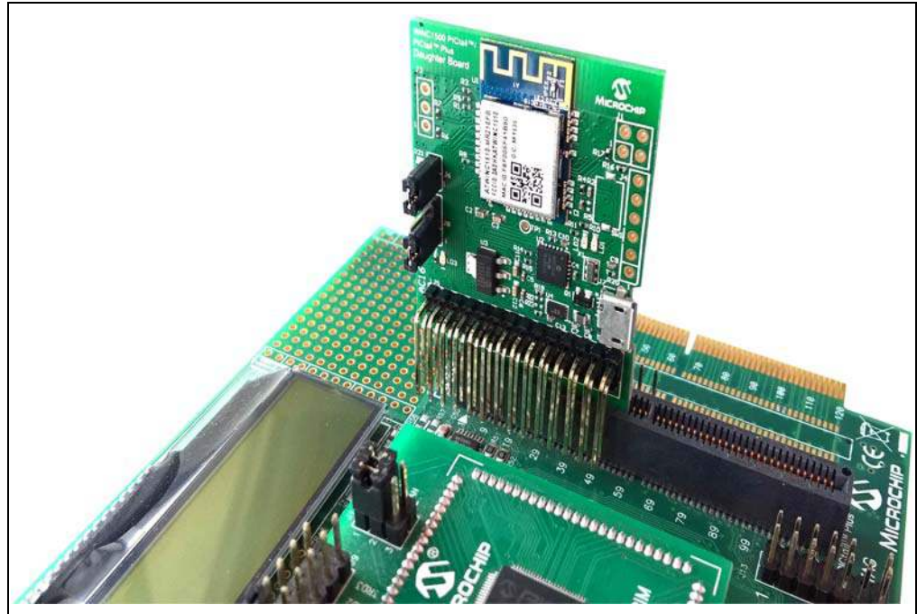
FIGURE 3-2: WINC1500 DAUGHTER BOARD PLUGGED INTO EXPLORER 16 DEVELOPMENT BOARD
