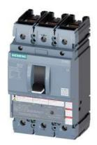
circuit breaker 3VA5 UL frame 250 breaking capacity class C 100kA @ 480 V 3-pole, line protection TM210, FTFM, In=90A overload protection Ir=90A fixed short-circuit protection Ii=10 x In UL489 SB (naval), 50 deg. cel. cable connection on both sides
