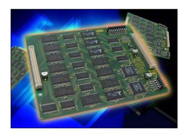
The Trace1 Board is available as an optional extra to ICPEIC3. It is a simple plug on connection to the motherboard.
