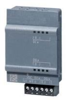
SIPLUS S7-1200 SB 1223 I/O based on 6ES7223-3BD30-0XB0 with conformal coating, -40...+60 °C, start up -25 °C, digital input/output 2 DI/2 DQ, 24 V DC 200 kHz
