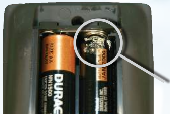
Corrosion you CAN see
