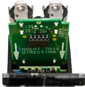
Figure 2. Q45 battery board
