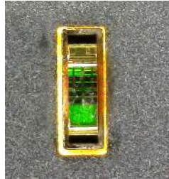
Figure 9-5. Image of FPCB With OPT4001 Mounted, Receiving Light Through the Cutout with a Rectangular Shape
