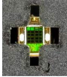
Figure 9-4. Image of FPCB With OPT4001 Mounted, Receiving Light Through the Cutout with a Plus Shape
